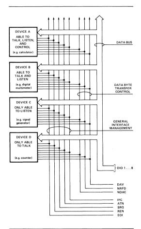
Figure 1. Interface Capabilities and Bus Structure.
